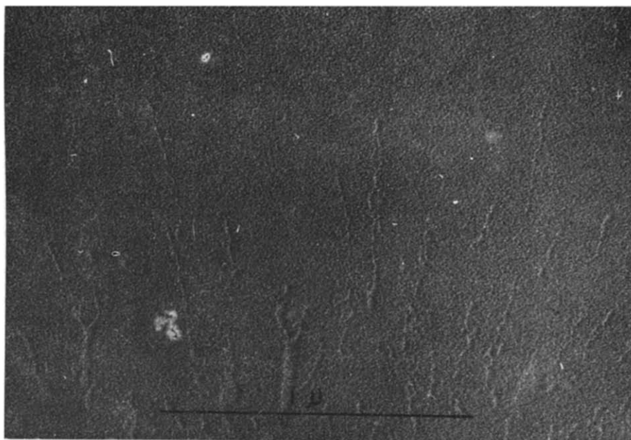
Fig. 2. E. coli RNA in water solution sprayed from low pressure gun and air-dried at room temperature. Shadow cast with Pt at a shadow to height ratio of 6:1.
